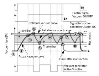
Fig. 9: Vacuum/signal curves
