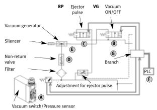
Fig. 10: Block diagram for VADMI-...\_LS
