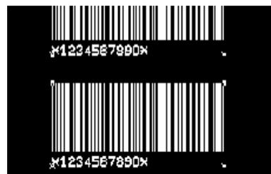
You can clearly notice from the above-mentioned example that the consumption of transfer ribbon is much lower when using the mode ribbon saving.
