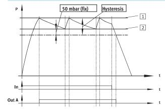
If the desired threshold 1 is reached for the vacuum, vacuum generation is automatically switched off. A nonreturn valve prevents the reduction of the vacuum.
