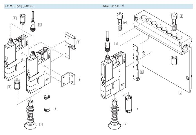
1) Hollow bolt 9 and mounting bracket 10 are included in the scope of delivery of the OVEM-...-PL/PO-....
