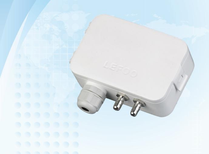
LFM108 differential pressure transmitter detect differential pressure or gauge pressure then convert this pressure difference to a proportional analogue output signal. Two output version are offered: Voltage output of  $0\sim10\mathrm{VDC}$ , and a current output 4-20mA. LFM108 differential pressure transmitter ranges from  $0\sim\pm50\mathrm{Pa}$  to  $0\sim\pm10000\mathrm{Pa}$ . These transmitters boast of their outstanding performance, high quality and economical pricing.
