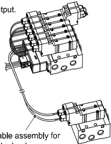
Cable assembly for output entry (EX510-V□□□)
