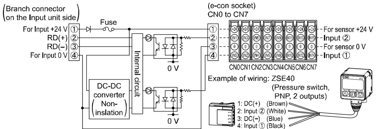
•EX510-DXN2: Input unit for NPN (1 connector 1 input type)
