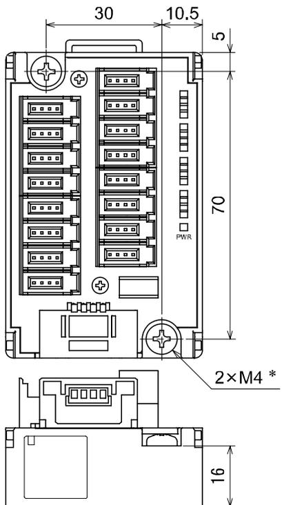
Cover removed (tolerance  $\pm 0.2$  mm)
