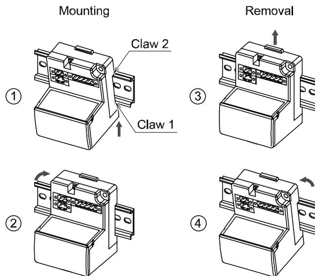
Put claw 1 of the body under DIN rail and push it upward. Push down Claw 2 to the opposite rail until the claw clicks securely on to rail.
