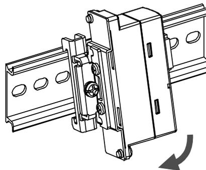
1, Hook claw 1 over the upper side and claw 2 over the low side of DIN rail respectively.
