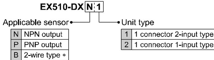
\*: B (2-wire type) is available with 1 connector, 2-input type only.
