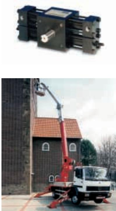
Telescopic access platforms demonstrate the real strengths of mobile hydraulics – a compact, self-contained power source; smooth, progressive power delivery and the inherent safety of the non-compressible fluid medium.
