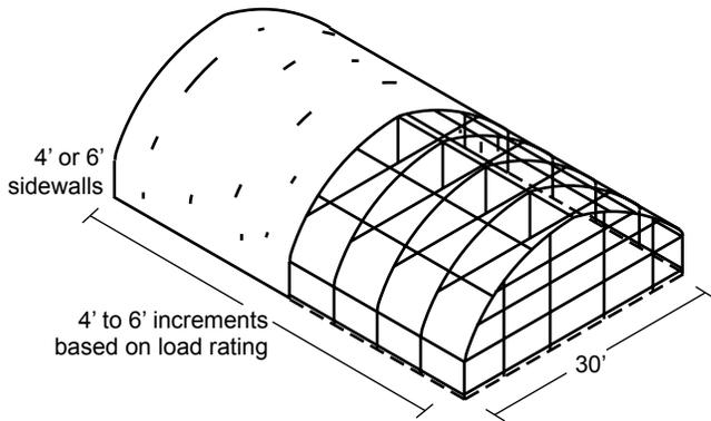
This greenhouse is engineered in accordance with Uniform Building Codes for almost any wind or snow load ratings. Stamped engineered plans can be provided at an extra cost. All galvanized steel frame insures maximum strength and life. Lexan polycarbonate covering is UV resistant with a 10 year discoloration warranty.
