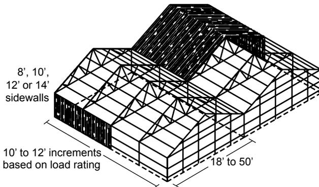
All Conley's greenhouses feature rollformed steel. Each truss assembly is made from one rollformed component, no splices required, between peak to gutter connection.
