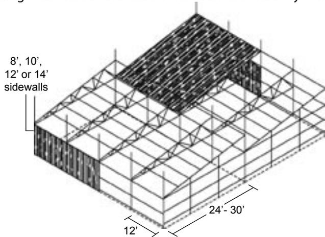
All Conley's greenhouses feature rollformed steel. Each truss assembly is made from one rollformed component, no splices required, between peak to gutter connection.
