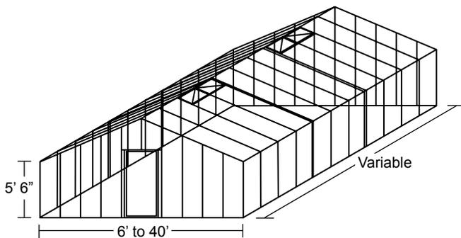
IGC glass greenhouses are also available with a curved eave and can be made to build on a knee-wall or glass to ground. Available in bronze, green or white. All IGC Glass Greenhouses are engineered to meet 80 mph wind and 30 pound live load per the UBC Building Code. For an additional expense, your structure can be designed to meet any building code requirements for live and/or wind load. Call IGC customer service for pricing on any custom requirements.
