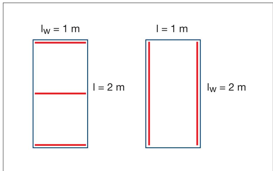
As we can see from this example, the length of a devifast™ fitting band may vary although the area and the distance between the devifast fitting bands remain the same
