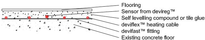
Thin floor on existing concrete floor - wet rooms
