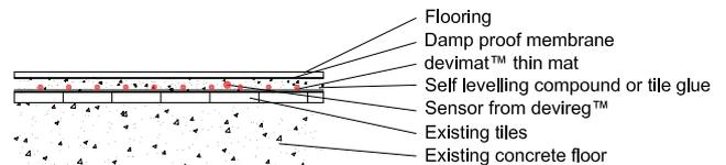
Thin floor on existing concrete floor - dry rooms
