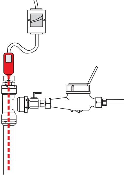
DTIV-9 (230 V, 9 W/m) and the devipeheat™ 10. The method is very efficient as the cable gets into direct contact with the substance to be heated.
