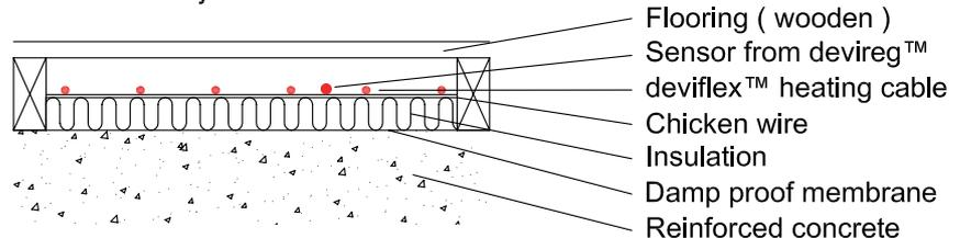
Renovated thin floor on wooden construction
