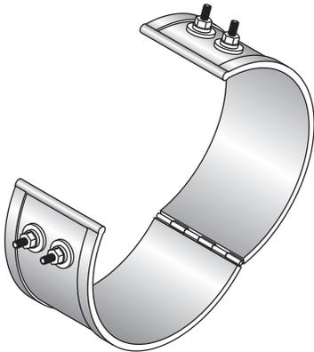
**Expandable or Hinged-** One piece construction used where heater cannot be slid over the barrel or die. Two sets of terminals required. All terminations available
