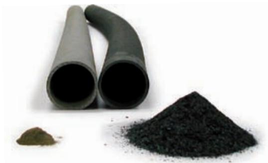
*Visual differences in oxide spallation and sagging properties between the tube Kanthal APMT (left) and a standard Fe-Ni-Cr tube after 2300 h at 1100°C (2010°F).*
