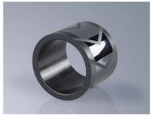
EKasic® Silicon Carbide laserstructured sliding bearings (left: radial bearing, right: thrust bearings) used e.g. in highly-loaded chemical pumps, in magnetic couplings for hermetically sealed pumps and in stirrers for chemical and pharmaceutical processes
