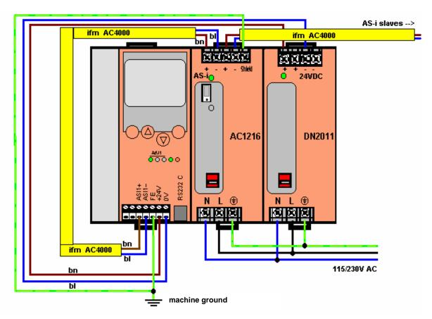
Figure: non binding suggestion for wiring of the controllere
