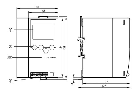
Figure: dimensions of the controllere
