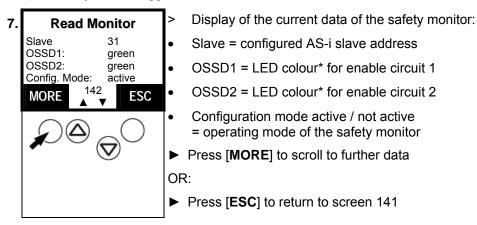
red = relay contact interrupted: safety device triggered
