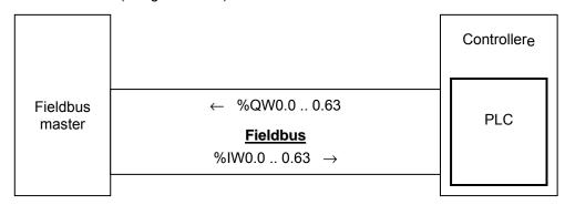
The output words %QW0...63 are sent by the PLC to the fieldbus master.
