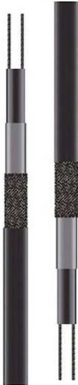
Self-regulating heating tapes consist of two parallel buswires, embedded semi-conductive self-regulating matrix. This means that the heating cable automatically responds to changes in ambient conditions.
