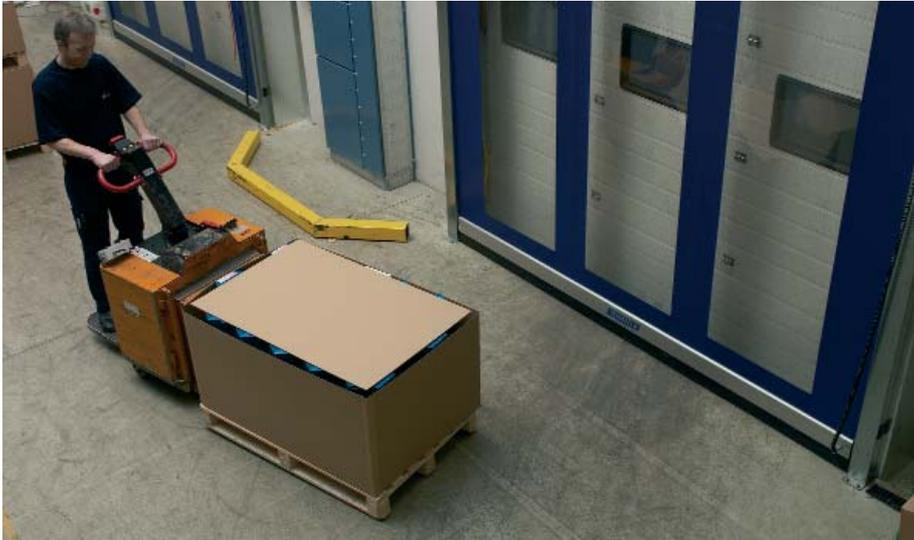
system should cover an area of min. 1 metre from the door and 0,5 metre to each side.
