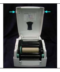
Push the front cover piece button inward to open. Lift/take off the front cover piece according to direction shown.
