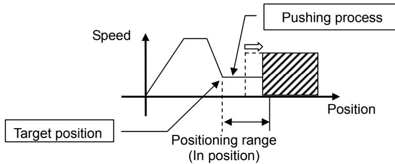
(2) Movement of the workpiece in the direction opposite to the pushing direction
