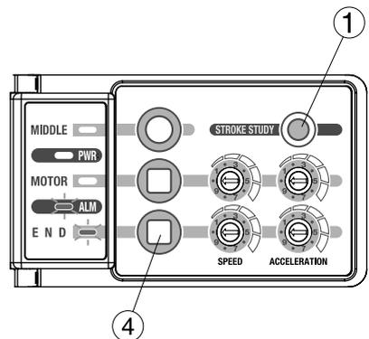
When changing the setting switch of speed and acceleration under locked condition, ALM indicator will blink.
