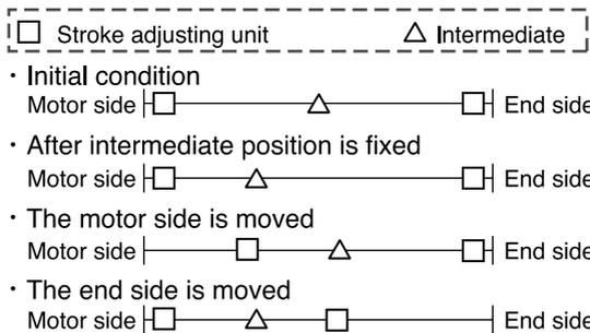
If the stroke is set shorter than the distance between the motor side and intermediate position, the intermediate position is fixed to the center of the stroke automatically.
