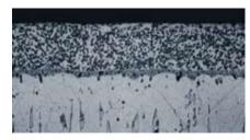
Cross section of EKatex® coating - electroless Nickel diamond dispersion (2  $\mu m)$
