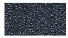
SEM image of EKatex® coating - electroless Nickel diamond dispersion (2  $\mu\text{m})$
