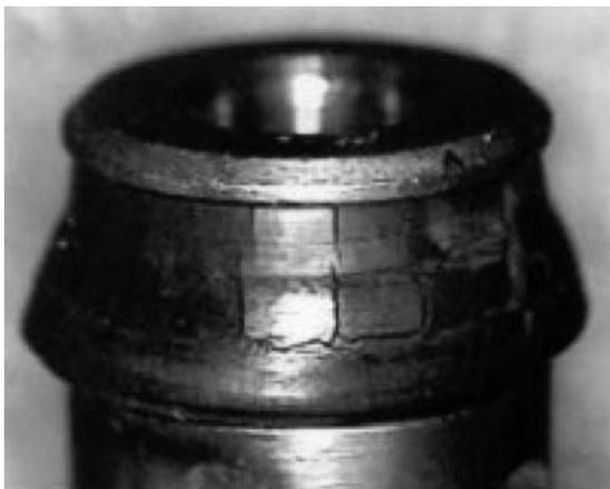
Photo 2 Cracking of check valve seal
