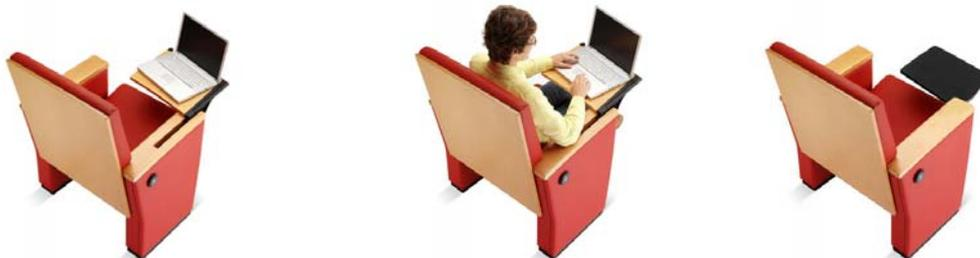
The seat is with the same characteristics as the back, but with only one block of foam. The seat folds automatically by a double lateral ball-and-socket joint of nylon (tested at 120.000 cycles), which operates without sound and requires no maintenance. The frontal part of the seat shows a perforated superficial in order to improve the acoustical absorption using a Helmholtz system.
