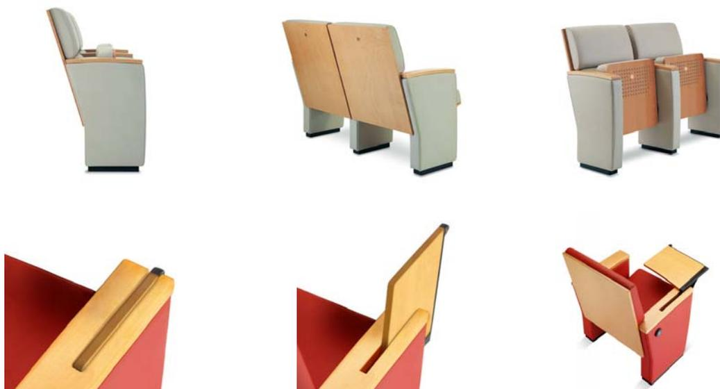
Seat designed with special acoustical characteristics for use in auditoriums and conference halls. The rear of the back is made of 15-mm thick beech wood covered in the front with two blocks of open cell polyurethane foam with special acoustic properties. The lower cushion is for lumbar support and the upper one support the cervical vertebrae. All this, together with its generous dimensions, gives a high level of comfort even during long periods of use.
