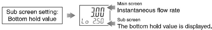
The maximum (peak) and minimum (bottom) flow from when the power is supplied to this moment is detected and updated.
