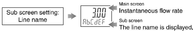
The name of piping line at which the product is installed can be displayed. Refer to [F82] Input of line names on page 51 for how to input the line name.
