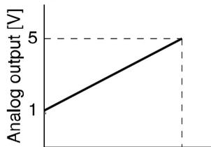
Min. rated flow    Max. rated flow
