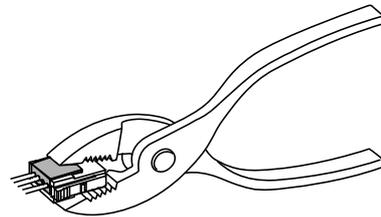
(It checks that the above-mentioned preparation work has been performed correctly, and A part shown in right figure is pushed by hand and makes temporary connection.
