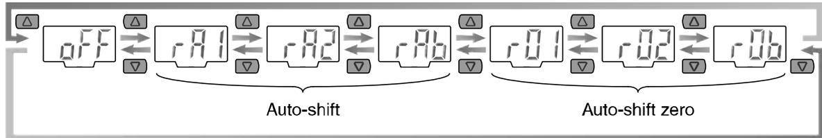
The setting of selected output is initialized when switching the selection of the external input.
