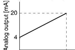
Min. rated flow    Max. rated flow
