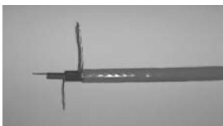
3. Now, remove the outmost 20 mm of the primary insulation. Use knife. Cut up the core material along one of the conductors and release it.
