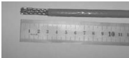
1. Remove 30 mm of the heating cable outer sheath.
