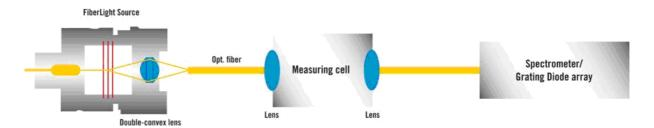
With plano-convex lens for direct illumination of measurement cell
