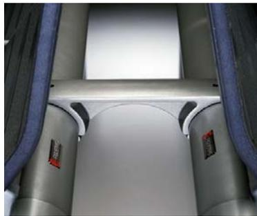
A modular bench of generous dimensions and special ergonomic characteristics essentially defined by its individual metal seating covered with open-cell polyurethane foam cushions with a TS fire curtain and vinyl covering. Each assembly comprises a frame consisting of four feet and a double link bar to which the seats are attached. All the structural components are made of aluminium and there are no welds in the whole assembly, which prevents rusting and ensures easy maintenance.
