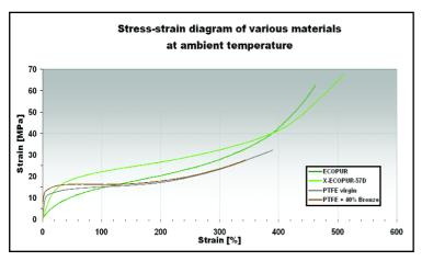
Fig. 8: Stress-strain graphs of sealing materials
