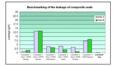
Fig. 17: Leakage characteristics of commercially available composite seals compared to X-ECOPUR®-57D
