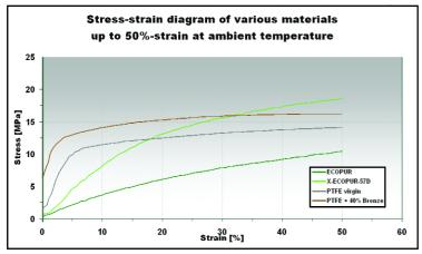
Fig. 6: Stress-strain graphs of various sealing materials
