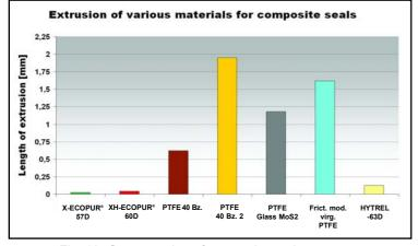
Fig. 13: Gap extrusion of composite seals
