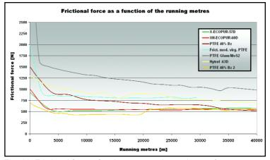
Fig. 11: Frictional force of various composite seals as a function of the running metres.
