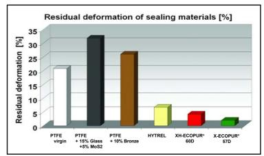
Fig. 10: Tensile set of various sealing materials
