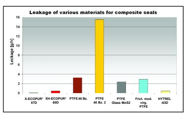
Fig. 12: Leakage of composite seals
