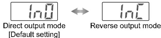
2)The operating mode and the output style for OUT2 is set. (only CH1)
