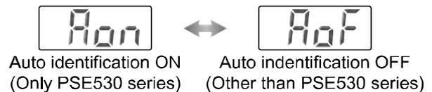
\*: Setting for the automatic identification function is ON when default setting.
