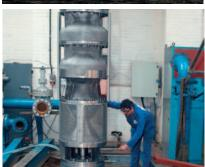
Designed to complement the **Hayward Tyler** motor range, our submersible solutions offer a comprehensive choice for the materials of construction. The pump duty is matched to customer requirements by selecting the pump size, number of stages and trimming the impellers. The applications are usually seawater lift or firewater pumps. The pumps are supplied, fitted to and powered by a submersible motor.
