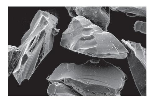
TETRABOR® boron carbide is a high-performance abrasive with a hardness and chemical resistance comparable to that of diamond. Thanks to its extreme hardness, TETRABOR® is often known as "black diamond," and is ideal for machining hard materials by lapping, sawing or ultrasonic drilling.
