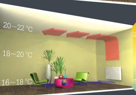
Convection in a room heated by a radiator
