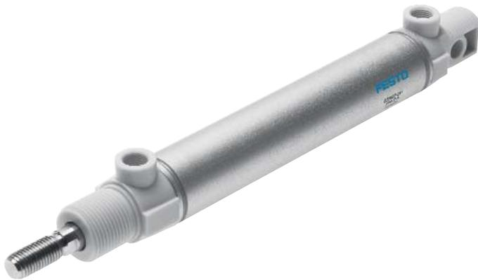
**DSNUP-....-P-A** with position sensing and flexible end position cushioning. Threaded bearing cap, end cap with swivel mounting and thread to ISO 6432
