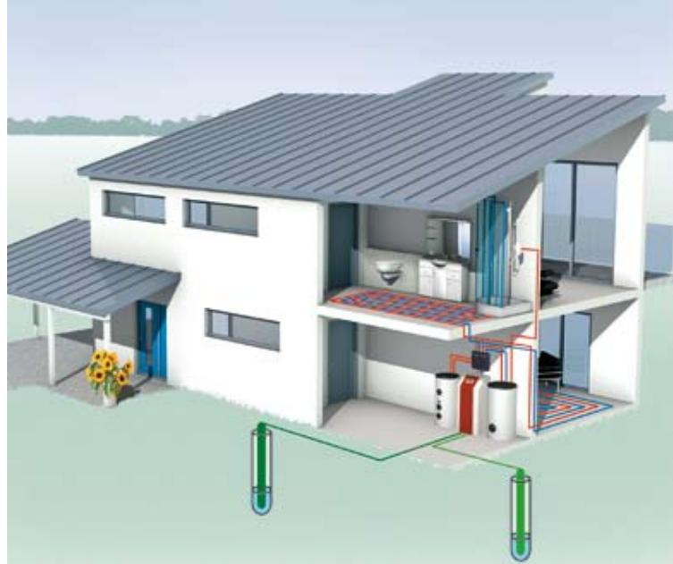
Water-to-water heat pump with well system
