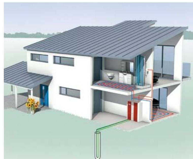
Brine-to-water heat pumps with borehole heat exchangers
