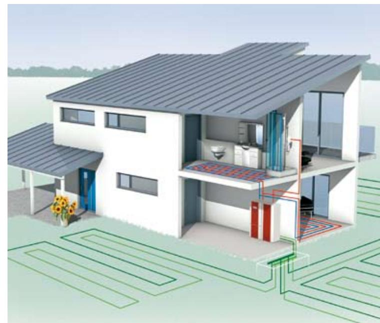
Brine-to-water heat pumps with ground heat collectors
