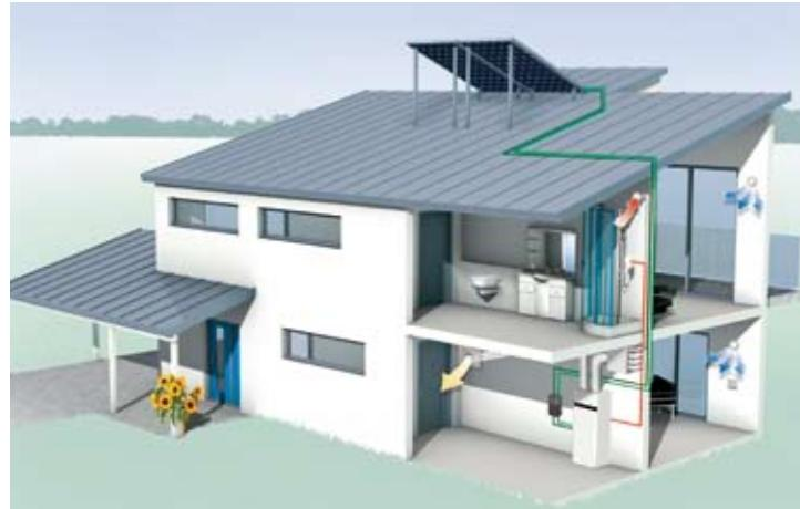
Solar collectors in combination with LWP 300W compact domestic ventilation unit
