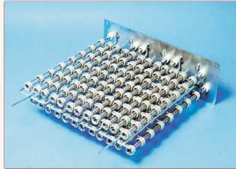
Our open frame duct heaters are very rugged and efficient air heaters. They are designed to heat large volumes of air in ducts. The open designs provide very low pressure drops across these heaters. Our low static pressures allow customers to use smaller and more economical blowers since there is little restriction of air flow. Systems can be more efficient.
