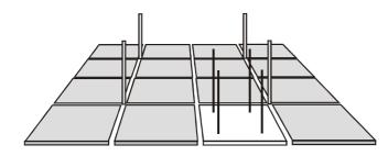
Cassettes are installed within a suspended ceiling construction. For additional support the cassette may be suspended independently within the grid.
