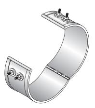
**Expandable or Hinged-** One piece construction used where heater cannot be slid over the barrel or die. Two sets of terminals required. All terminations available
