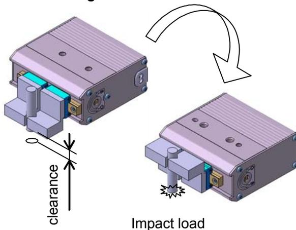
**9. When mounting a work piece, align it with the product carefully to prevent excessive force to the finger.**
