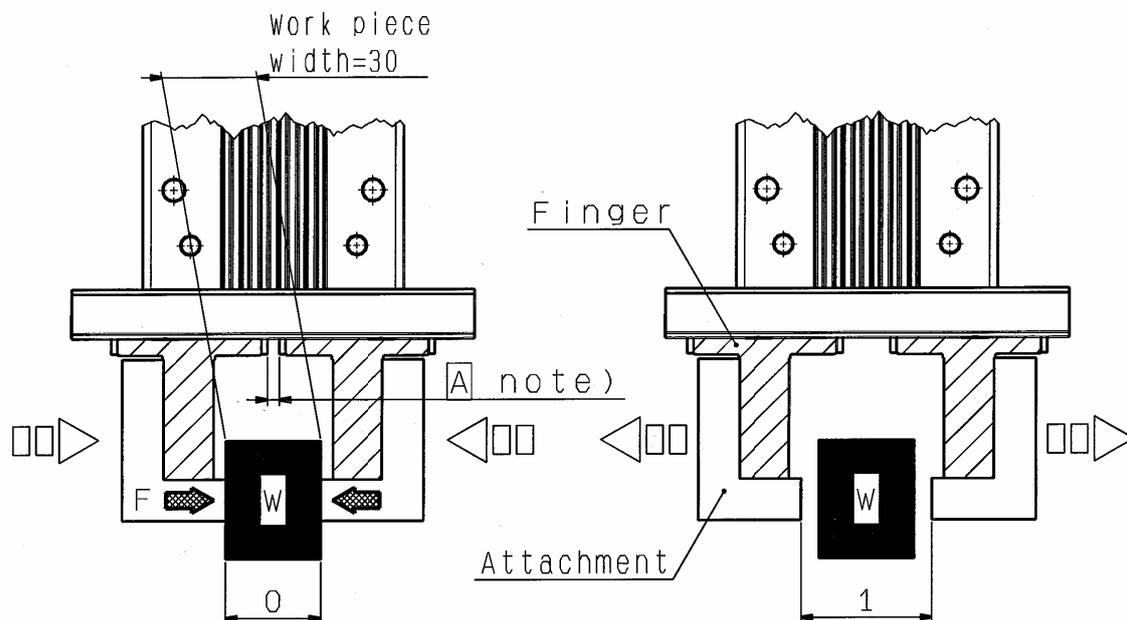
Note) When the work piece is used to define the origin, the stroke (moving distance) will be shortened by  $A$  mm, so check the step data again.
