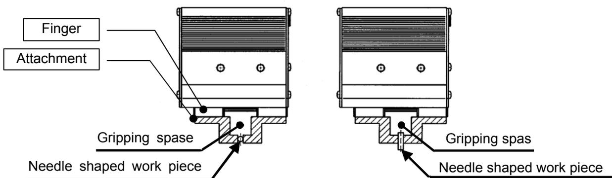
4. **Select the model that allows for gripping force in relation to the weight of a work piece, as appropriate.**
