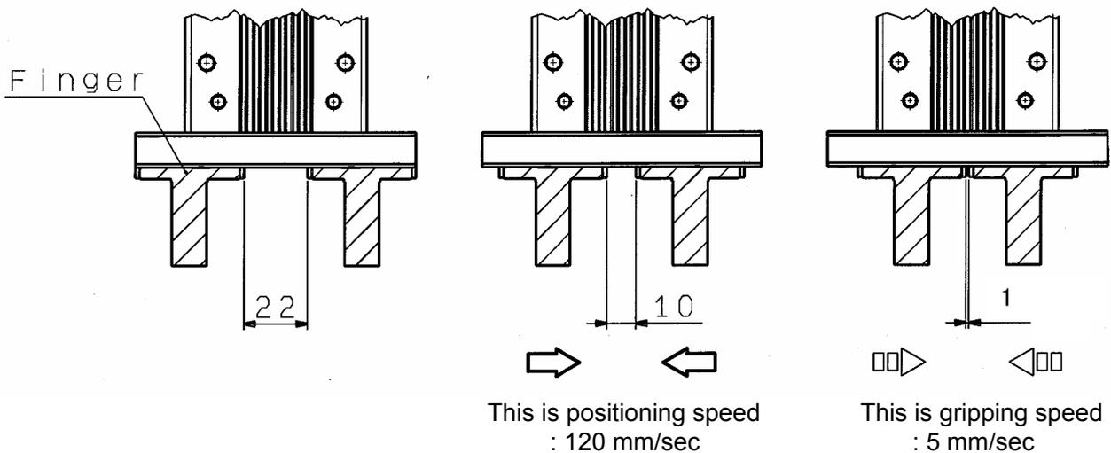
Condition 2) In case the pushing operation is **Step no. 1** to **Step no. 2**
