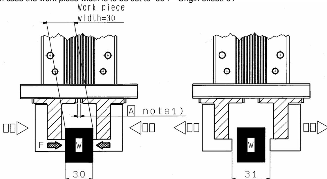
Note 1) If the work piece is used to define the origin, the stroke (moving distance) will be shortened by  $A$  mm, so check the step data again.
