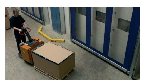
system should cover an area of min. 1 metre from the door and 0,5 metre to each side.
