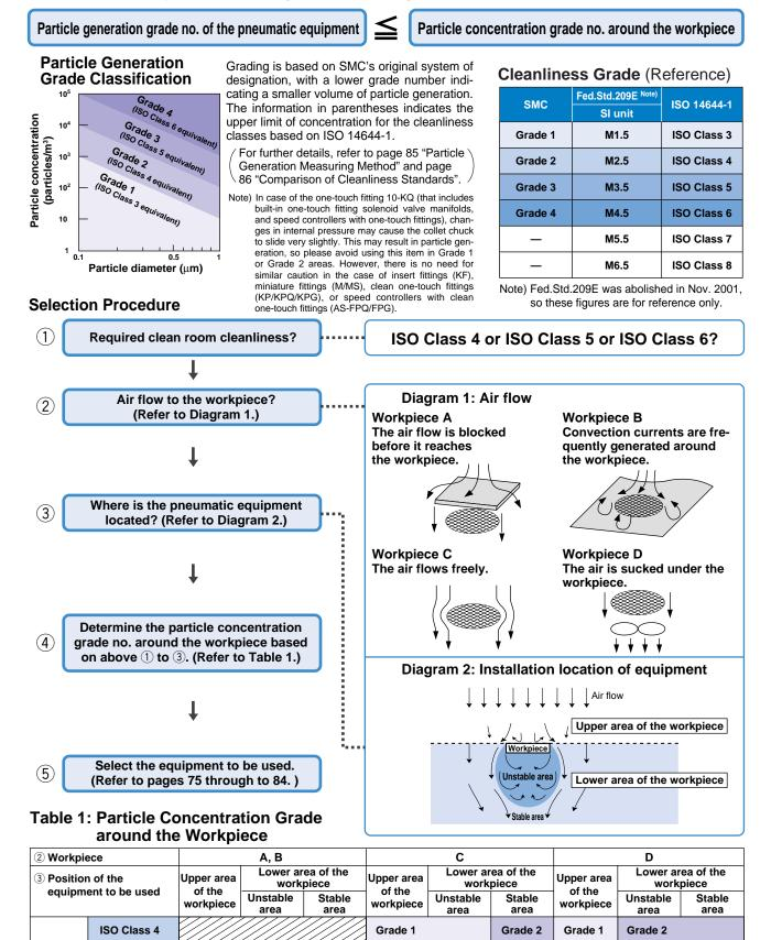
ISO Class 4 and 5 levels of cleanliness cannot be achieved in area due to dust accumulation or flotation.
