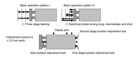
e-Rodless Cylinder Series E-MY2 Low speed (Intermediate stop) Shock relief
