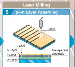
A laser is used to cut p-i-n layers to form circuits.
