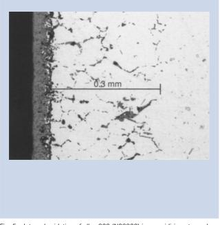
Fig. 5 – Internal oxidation of alloy 800 (N08800) in an oxidizing atmosphere at 980 °C (1796 °F) after 10,000 hrs.
