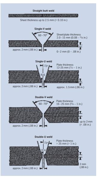
Fig. 10 – Edge preparation for welding of nickel alloys and special stainless steels.
