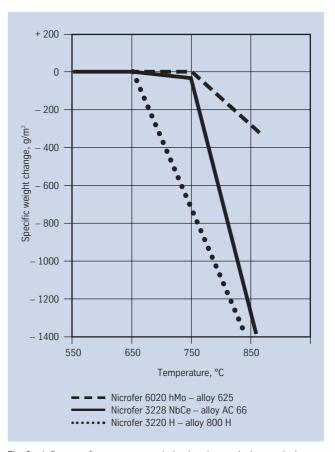
Fig. 9 – Influence of temperature on behaviour in a typical waste incineration atmosphere under cyclic conditions: Comparison of specific weight change in a simulated waste incineration environment consisting of nitrogen with 9%  $O_2$ , 2.5 g/m<sup>3</sup> HCl and 1.3 g/m<sup>3</sup> SO<sub>2</sub> after 1000 hrs cyclic exposure at temperatures of 550 to 850 °C (1022 to 1562 °F).
