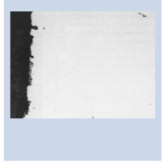
Fig. 6 – Nicrofer 3228 NbCe without evidence of internal oxidation in an oxidizing atmosphere at 980  $^\circ$ C (1796  $^\circ$ F) after 10,000 hrs.
