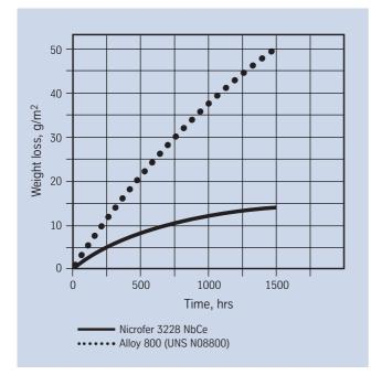
Fig. 8 – Comparison of weight loss of Nicrofer 3228 NbCe and alloy 800 in an  $H_2/H_2O/HCI$  atmosphere at 900 °C (1652 °F) after 1500 hrs.
