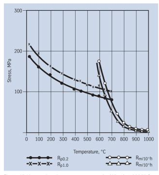
Fig. 1 – Yield strength and creep-rupture strength of Nicrofer 3228 NbCe.
