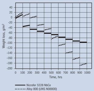
hrs Time, hrs Nicrofer 3228 NbCe ...... Alloy 800 (UNS N08800) the weight loss of austenitic Fig. 4. Weight loss comparison in air at 980 °C (
