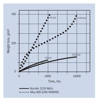
Fig. 7 – Comparison of weight loss of Nicrofer 3228 NbCe and alloy 800 respectively in high- and low-sulfur containing process gases at 940 °C (1724 °F) after 10,000 hrs.
