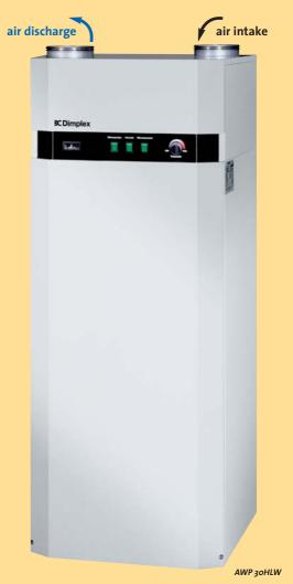
With the AWP 30HLW heat pump water heater, Dimplex offers the compact residential heat recovery ventilation system LWP 300 W (exhaust air volume flow settings: 230/185/120 m3/h). Building ventilation is effected via a 2-pipe residential ventilation system with central exhaust air and decentralised outside air supply systems via outdoor wall valves.
