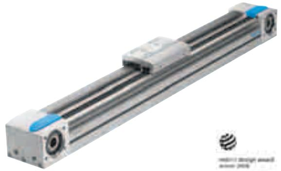
**The electric linear axis EGC with recirculating ball bearing guide: maximum dynamic response and speed with improved rigidity.** Toothed belt drive for maximum dynamic response or spindle drive for high precision; suitable for all motor types.
