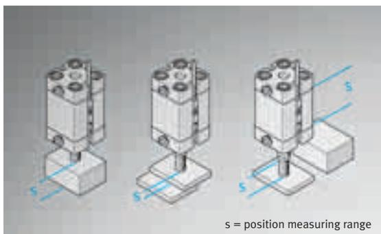
Simple measurement of position in a defined area
