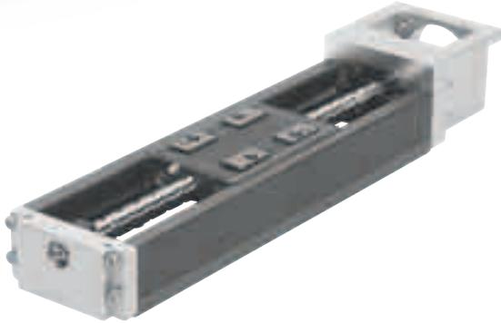
**For highly precise and space-saving applications: linear axes EGSK and EGSP.** The EGSK version comprises a spindle axis with recirculating ball bearing, and EGSP has a spindle axis with an innovative caged ball chain. Both have an extremely compact design. Spindle axis and recirculating ball bearing guide – the proven principle for precision and excellent running characteristics.
