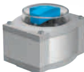
**Complete, reliable, perfect fit.** The analogue position indicator reads out a 4 to 20 mA output signal and is used to monitor the positions of quarter-turn actuators. Not just the end positions, but rather the entire swivel angle range is indicated by the analogue signal output.
