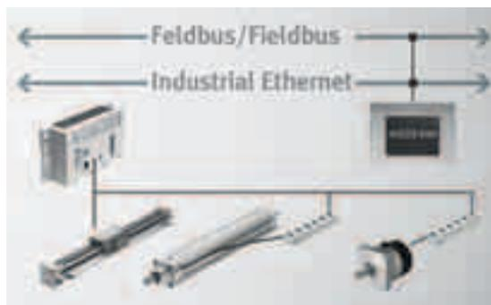
Different drives and displacement encoders – uniform system architecture
