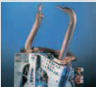
Efficient technology mix: servo-pneumatic welding tong with roughly 25% less compressed air consumption than conventional welding tongs
