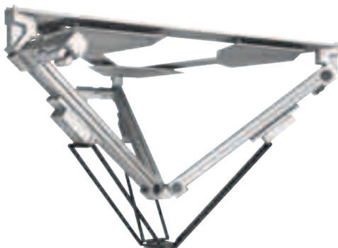
**Tripod kinematics enables free motion in 3D space. Ideal for high-speed handling of loads of up to several kilograms.** The setup consists of three securely mounted linear axes in the form of a closed pyramid and offers good rigidity and stability with minimal moving loads. This concept guarantees high dynamics with large effective loads.
