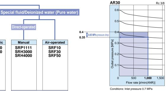
When the flow rate is 1,000  $\ell$ /min (ANR) with the outlet pressure set to 0.4 MPa, the outlet pressure goes down (pressure drop) to 0.35 MPa due to the flow characteristics. The guideline of pressure drop should be set to less than
