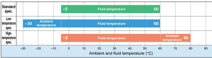
Note) The above indicates the temperature specification of a basic regulator for general purposes and a precision basic regulator. The standard temperature specification of an electronic regulator is ranging from 0 to 50°C.
