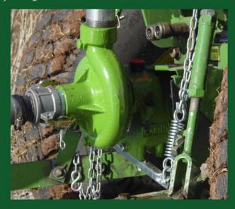
Rovatti T0F50 pumps are an extremely easy, portable, user friendly pump which can be directly attached to the PTO of most any 540 RPM tractor. Whether to fill ponds, sprinkler irrigate, wash down, transfer or tank filling, the T0F50 provides the solution inexpensively. The pumps provide up to 150 GPM and pressure as high as 75 PSI. The units come standard with a foot valve, suction and discharge fitting. These units are available in either standard centrifugal or self priming models.
