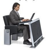
When folded away, the table and column assembly takes up just 190 mm. The table is opened by means of a simple, intuitive up-and-twist movement. This gives the user an ample working surface. The table has an anti-panic fold-away mechanism. This means that when the user gets up from the seat, this movement sends the table into the fold-way position, so that the hall is vacated quickly and the aisles are always left clear.
