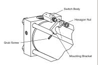
Fig. 4 Attaching a Read.me switch to bracket and tie rod
