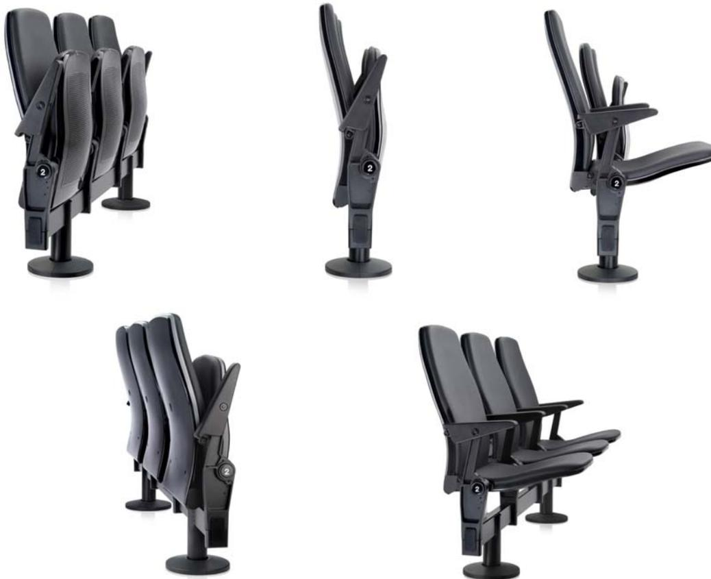
A beam-mounted, foldaway chair. The seat tips up, the back reverts to an upright position and the armrests fold up out of the way in a single, automatic movement. The seat tips up about its axis while the backrest moves forward until they are flat against one another. When folded away, the depth of the seat and backrest together is 245 mm (9.7"). As the seat and backrest fold away, the
