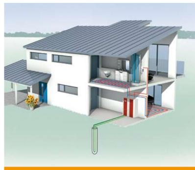
Brine-to-water heat pumps with borehole heat exchangers
