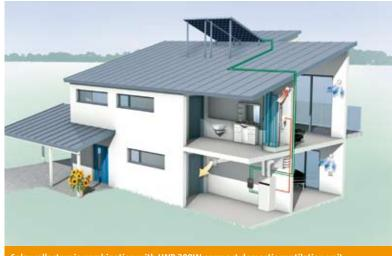
Solar collectors in combination with LWP 300W compact domestic ventilation unit with integrated DHW preparation
