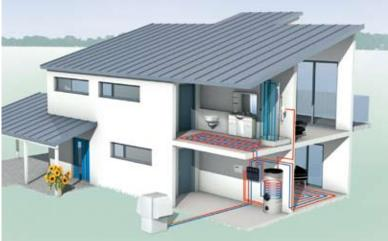
Air-to-water heat pumps for outdoor installation
