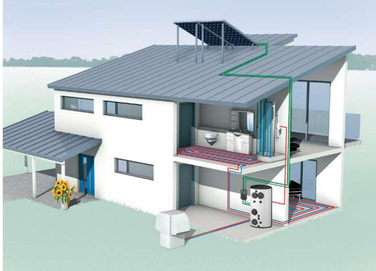
Solar collectors for domestic hot water preparation and supplementary heating in combination with air-to-water heat pumps
