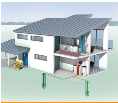
Water-to-water heat pump with well system
