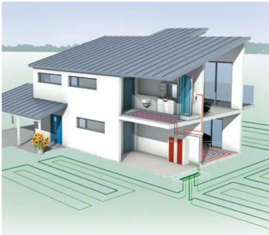
Brine-to-water heat pumps with ground heat collectors
