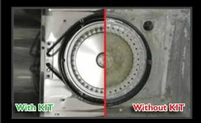
It is well-known that the presence of lime scale, minerals and other water impurities produce scale on the heating elements, ferrous residuals in the cavity, scale on the fans, with consequent loss of balance and problems for the motors. All this will result in a reduced life of the oven.
